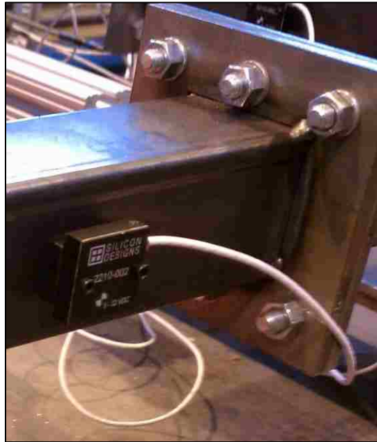
Figure 4.9: Model number 2210-002 produced by Silicon Design, Inc. (2010) Courtesy of E. Labuz 2011
